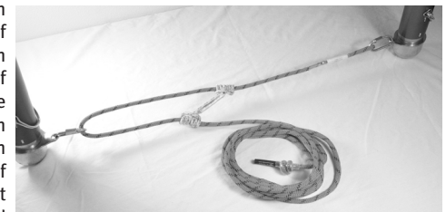
Fig 14 Rope Hobble Loop with Prussic. Sewn loop connected to quick link; large loop connected to 2nd leg quick link.
