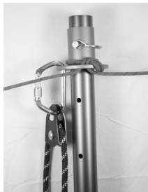
Fig 25 Lash Ring atop of gin pole as main attachment
