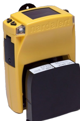
Fig. 4. Nardalert S3 mainframe shown with interchangeable sensor
